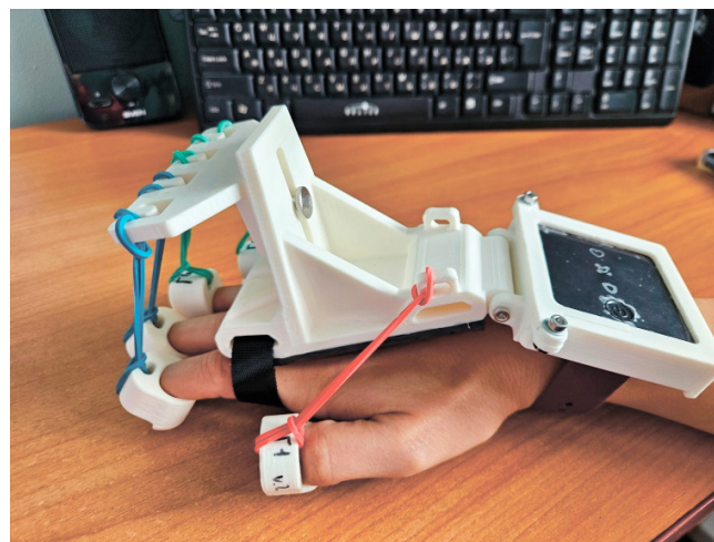
FIG. 1. Medical simulator "Glove" for correcting of upper limb spasticity
