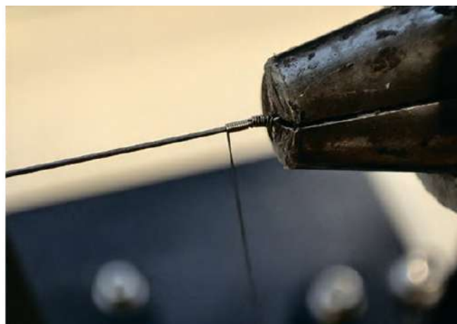
FIG. 1. Winding fixture for coil prototypes
